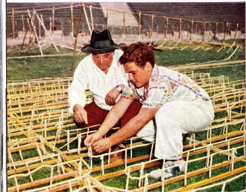
Lizza shows his son, Tiverio, the proper way to tie fuses to a frame that is rigged for a fireworks American flag.
