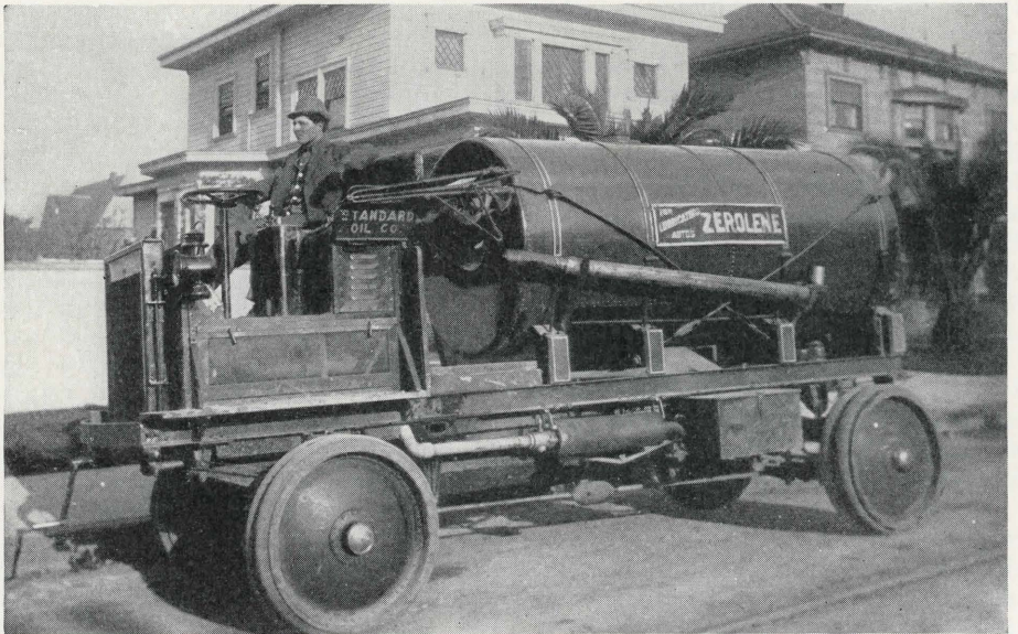
First motor-truck acquired by the Sales Department of the Company (in 1911) for delivering fuel oil. It was "couple-gear, motor-wheel-driven"—and self-starting on a down-grade
